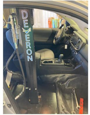
1: Deveron's automated soil probe and internalized sampling equipment increases the speed at which we can sample fields.
